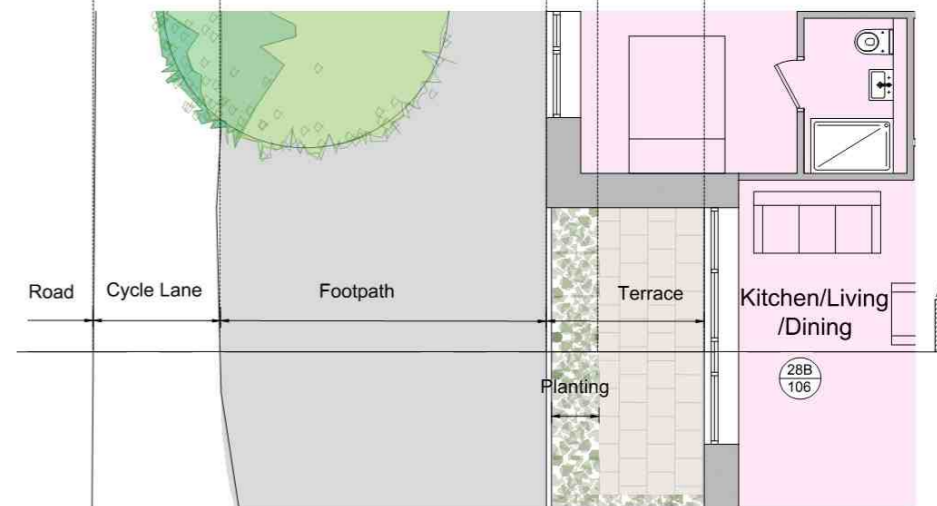
Threshold Condition 2, Block 28 - terrace raised above street level below
