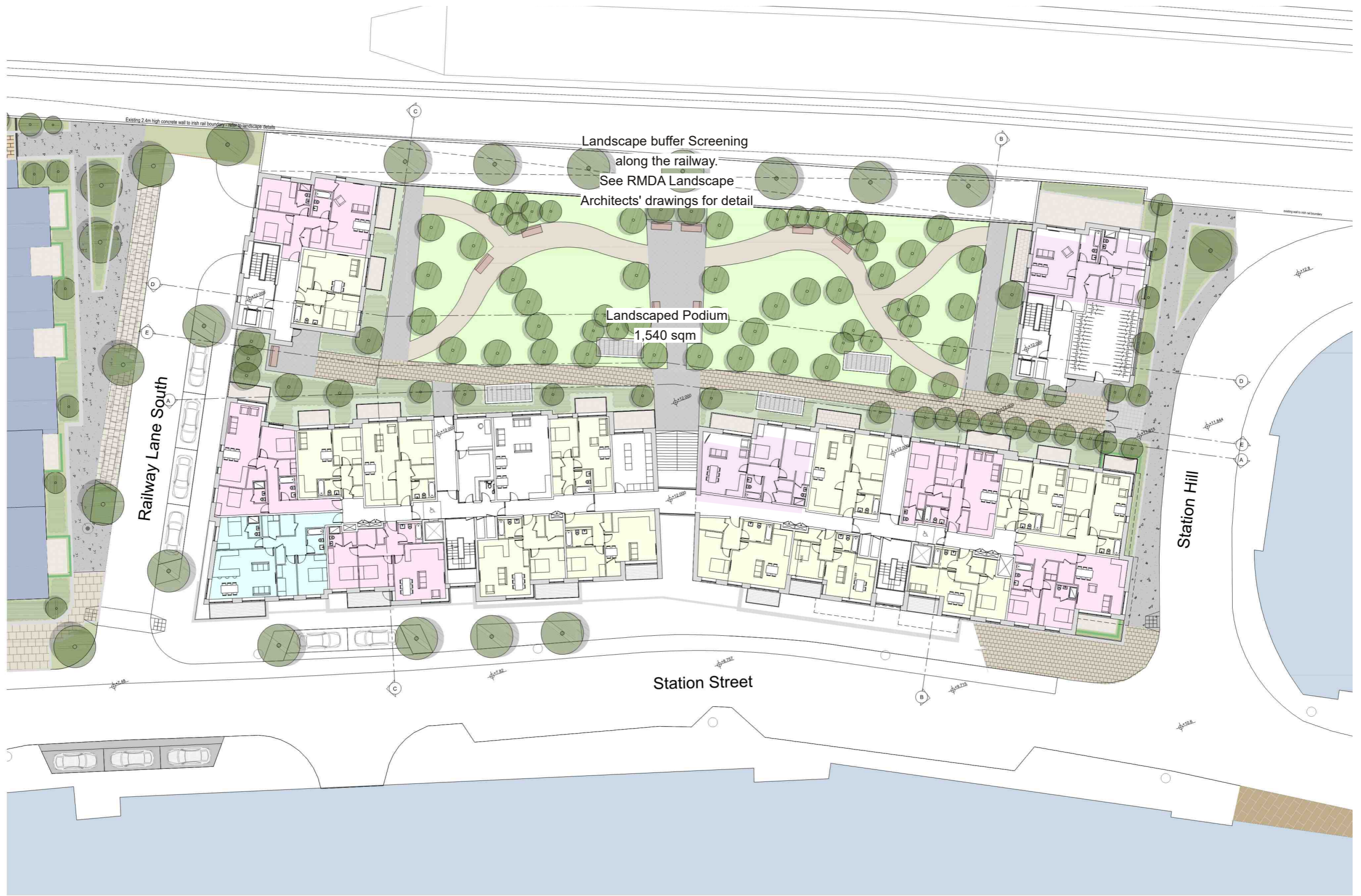
Communal landscaped courtyard at first floor podium level
